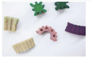
3D-PRINTING OF CELLULOSE BASED MATERIALS BY NSCRYPT METHOD
